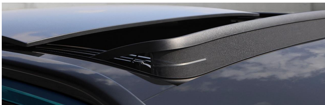
Techo cielo practicable
